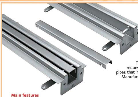
Particularly small channels made of 2 mm thick AISI 304 stainless steel for the drainage of water from balconies and terraces. The feature of a removable cover also makes it very convenient when it comes to cleaning. They are fitted with flanges along the perimeter to provide a perfect seal with the sealing gasket.
